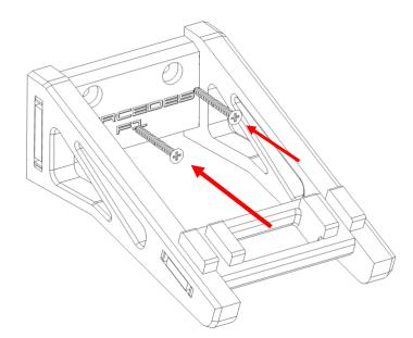
Install both screws into the back stretcher. Do not over tighten (use a screwdriver).
