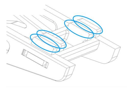
These tabs insert into the frame of the Lego set, Line up the tabs with the corresponding locations on the Lego set.
