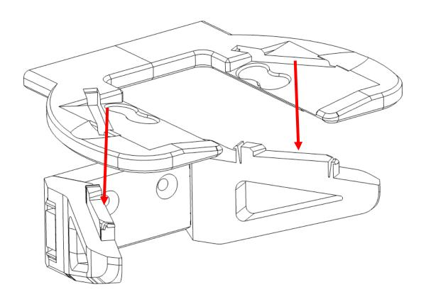
Use the provided wall fixings to secure to the wall. Do not over tighten the screws (use a screwdriver only).
